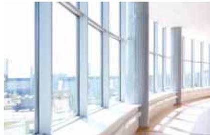
Color, finish and materials affect how light is reflected; unfortunately, they are rarely decided on at the time of the daylight modeling process. However, some assumptions can be made. A good rule of thumb is to assume 80% of light will be reflected by ceilings, 50% of light will be reflected by walls and 20% of light will be reflected by floors.
