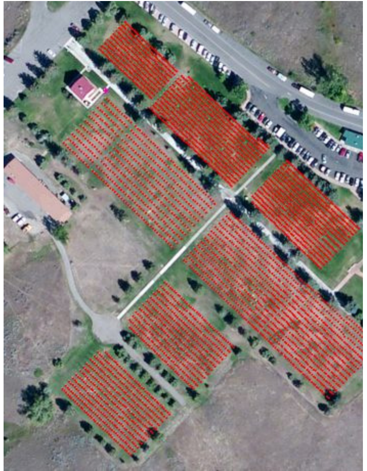
Cemetery markers at Little Bighorn were extracted from the high-density lidar data using Multi-Hill-shade Hierarchic Clustering (MHHC).
