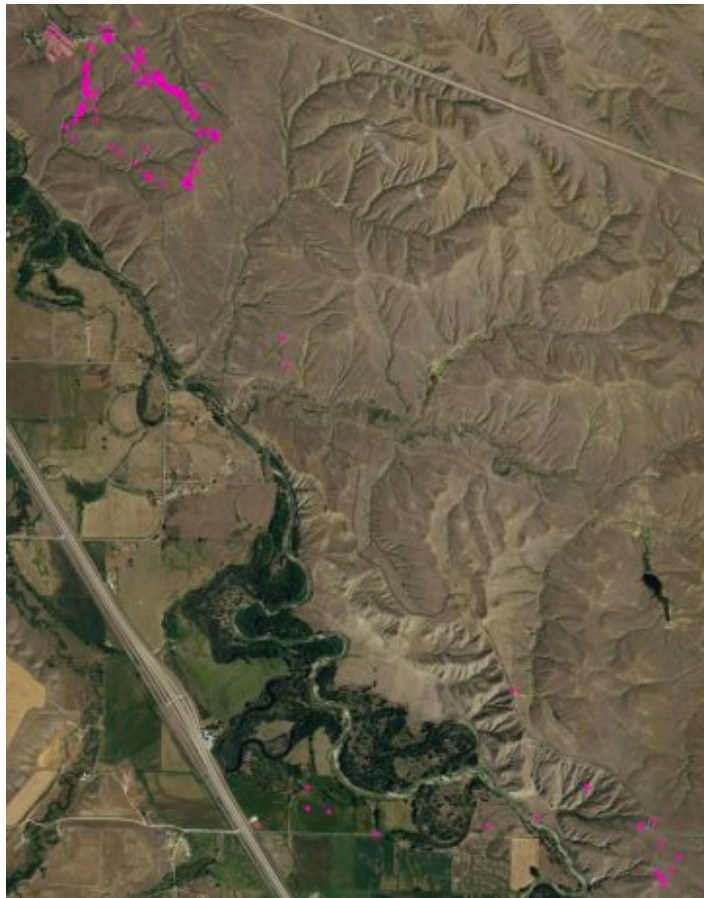
Battlefield markers also were extracted from the lidar data via MHHC, a three-step process that locates the center of gravity corresponding to the location of the marker.
