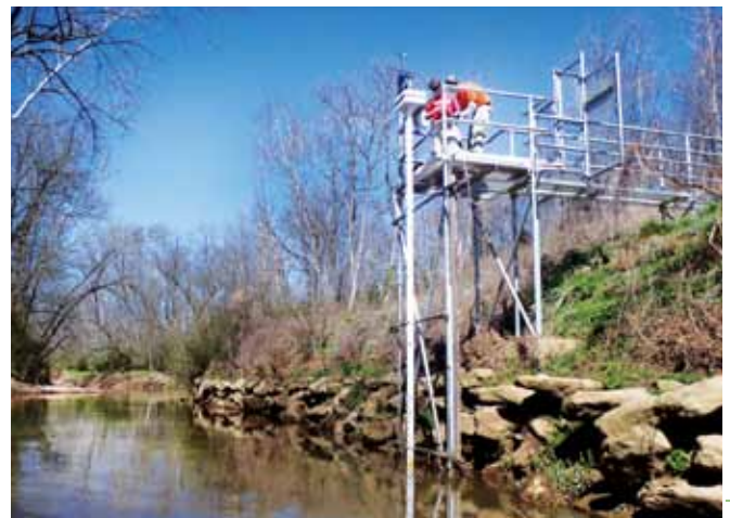
The permanent monitoring station features a stable aluminum platform that allows technicians to move over the body of water without getting wet.
