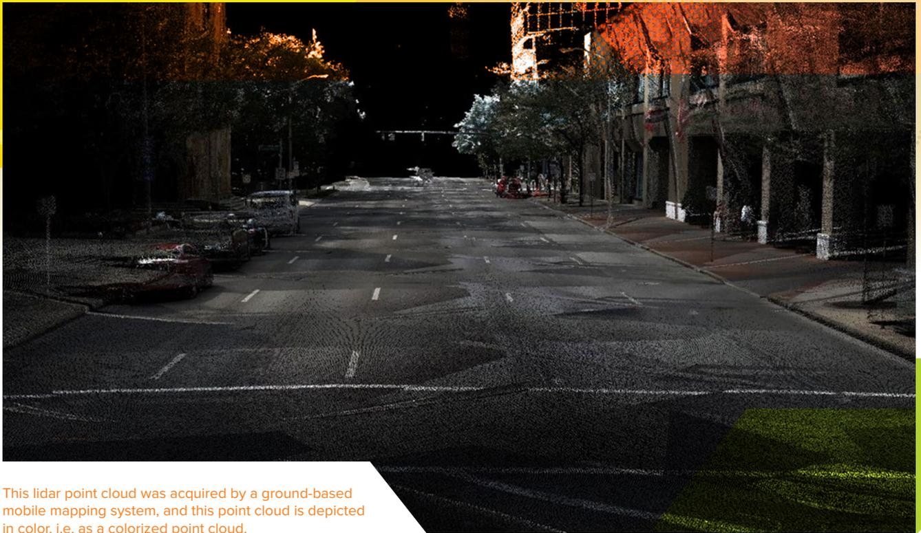
This lidar point cloud was acquired by a ground-based mobile mapping system, and this point cloud is depicted in color, i.e. as a colorized point cloud.
