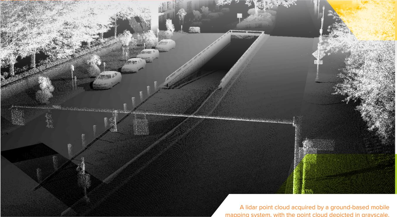
A lidar point cloud acquired by a ground-based mobile mapping system, with the point cloud depicted in grayscale.
