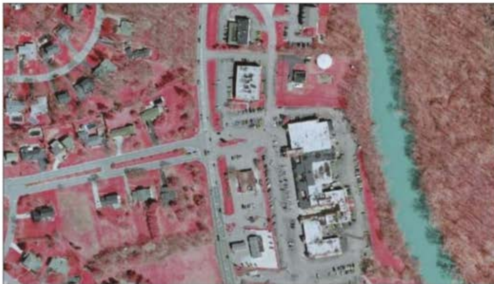
This color infrared image taken of Columbus, Ohio, illustrates digital ortho-imagery collected to determine accurate impervious surface area during the feature extraction method. (photo: Woolpert)
