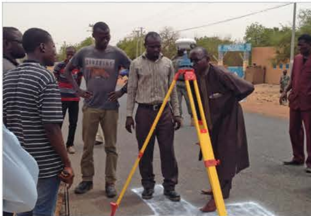
Cross-shaped targets were painted on pavement for the ground control survey if points fell on paved roadways. Courtesy of Woolpert
