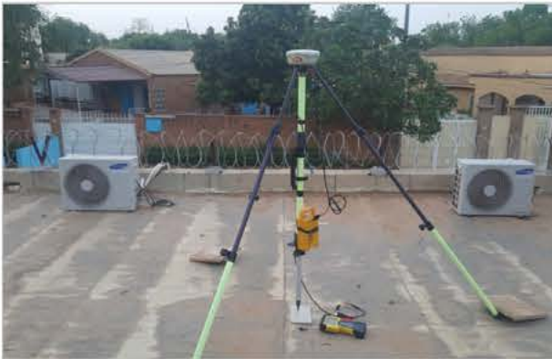
Each morning, a GPS base station was set up at designated locations in the survey area to support the ground control and aerial survey missions for the day. GPS base station data was collected once per second all day. Courtesy of Woolpert
