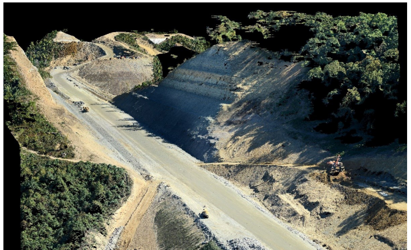
Figure 5. High quality points cloud from consumer grade camera imagery.
