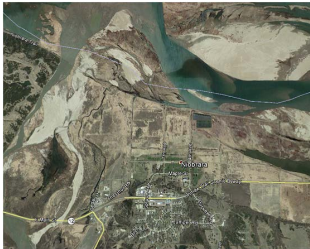
b. Lewis and Clark Lake, SD – Large sediment loads from tributaries have resulted in at least a 30% loss in total storage capacity (USACE, 2013). The upper reservoir is now so shallow that boats can be beached in the middle of the lake (upper left photograph) and the reservoir can be waded (lower left photograph). At least part of the City of Niobrara, NE had to be relocated because of the upstream growth of the sediment delta even though it was upstream from the reservoir pool (right photograph).
