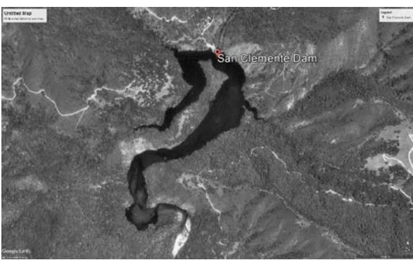
a. San Clemente Reservoir, CA – Photographs from Google Earth spanning two decades (1994 left and 2013 right) show the loss of reservoir storage capacity over time due to sedimentation.
