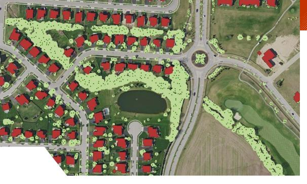
Building outlines, tree canopies and tree crowns, extracted from QL0 lidar, are represented in this screenshot. The Columbus (Ohio) **Recreation and Parks** Department, Urban Forestry Division, uses QL0 lidar data to produce canopy height and density models that estimate various measurements, such as a tree's crown and stem diameter or a forest's tree density and wood volume. Courtesy of Woolpert.
