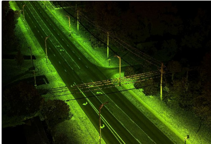
Figure 5: Mobile Lidar data over a portion of County Line Road in Dayton, Ohio. (Image courtesy: Woolpert)
