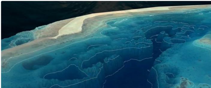
Figure 3: Satellite-derived bathymetry is used for filling gaps in this shallow water bathymetric survey. (Image courtesy: Satellite-Derived Bathymetry Technology and User Forum)
