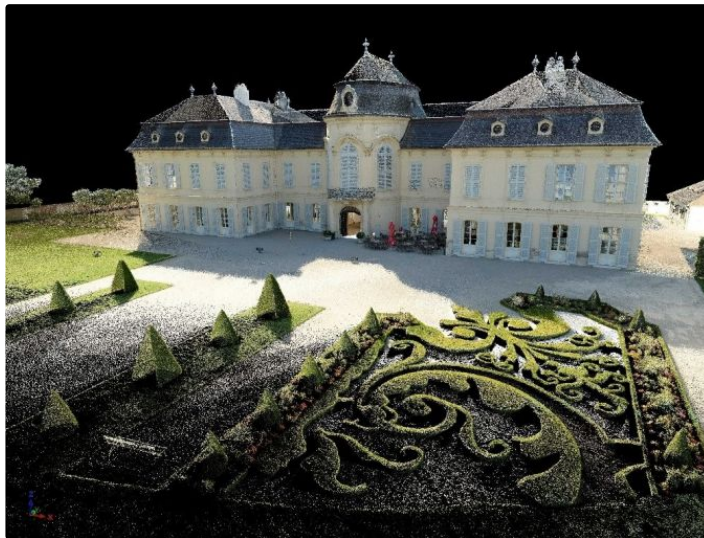
Figure 6: This colored exterior scan supports building information modelling. (Image courtesy: RIEGL)
