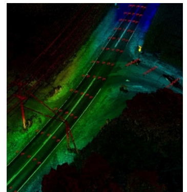
Figure 5: Point clouds from MMS (zone A) and the derived second-generation checkpoints
