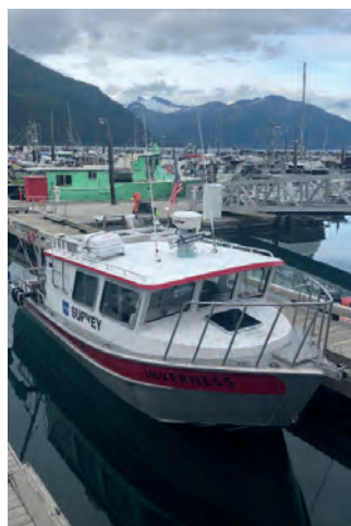
▲ For the project, the project team utilized an R2 Sonic 2024 multibeam echosounder which was mounted on the RV Inverness. The vessel was docked in Whittier Harbor during the project. (Image courtesy: Woolpert)
