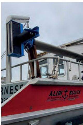
▲ For the project, the project team utilized an R2 Sonic 2024 multibeam echosounder which was mounted on the RV Inverness. The vessel was docked in Whittier Harbor during the project. (Image courtesy: Woolpert)
